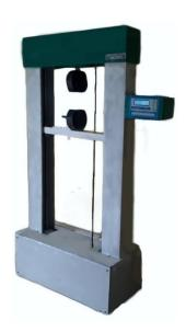
• Dumbbell Press offered by us are laboratory sample cutting presses that form an essential parts of laboratory. These are used primarily for cutting dumbbell shaped that are used in various tests like elongation test, tensile test and others. Further, type press has high impact hardened cutting screws that allows high volume cutting.
